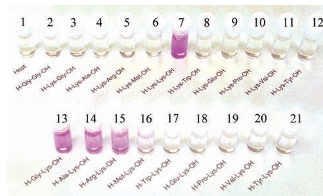
Figure 3. Visible recognition of the sequence of dipeptides by the host 1 . The concentration of 1 was 1.0 \times 10^{-3} M and those of dipeptides were 1.5 \times 10^{-3} in the presence of N -ethylpiperidine ( 2.5 \times 10^{-2} M) in methanol/water = 10/1. 1; Host 1 only, 2; Gly-Gly, 3; Lys-Gly, 4; Lys-Ala, 5; Lys-Arg, 6; Lys-Met, 7; Lys-Lys, 8; Lys-Trp, 9; Lys-Glu, 10; Lys-Pro, 11; Lys-Val, 12; Lys-Tyr, 13; Gly-Lys, 14; Ala-Lys, 15; Arg-Lys, 16; Met-Lys, 17; Trp-Lys, 18; Glu-Lys, 19; Pro-Lys, 20; Val-Lys, 21; Tyr-Lys.
